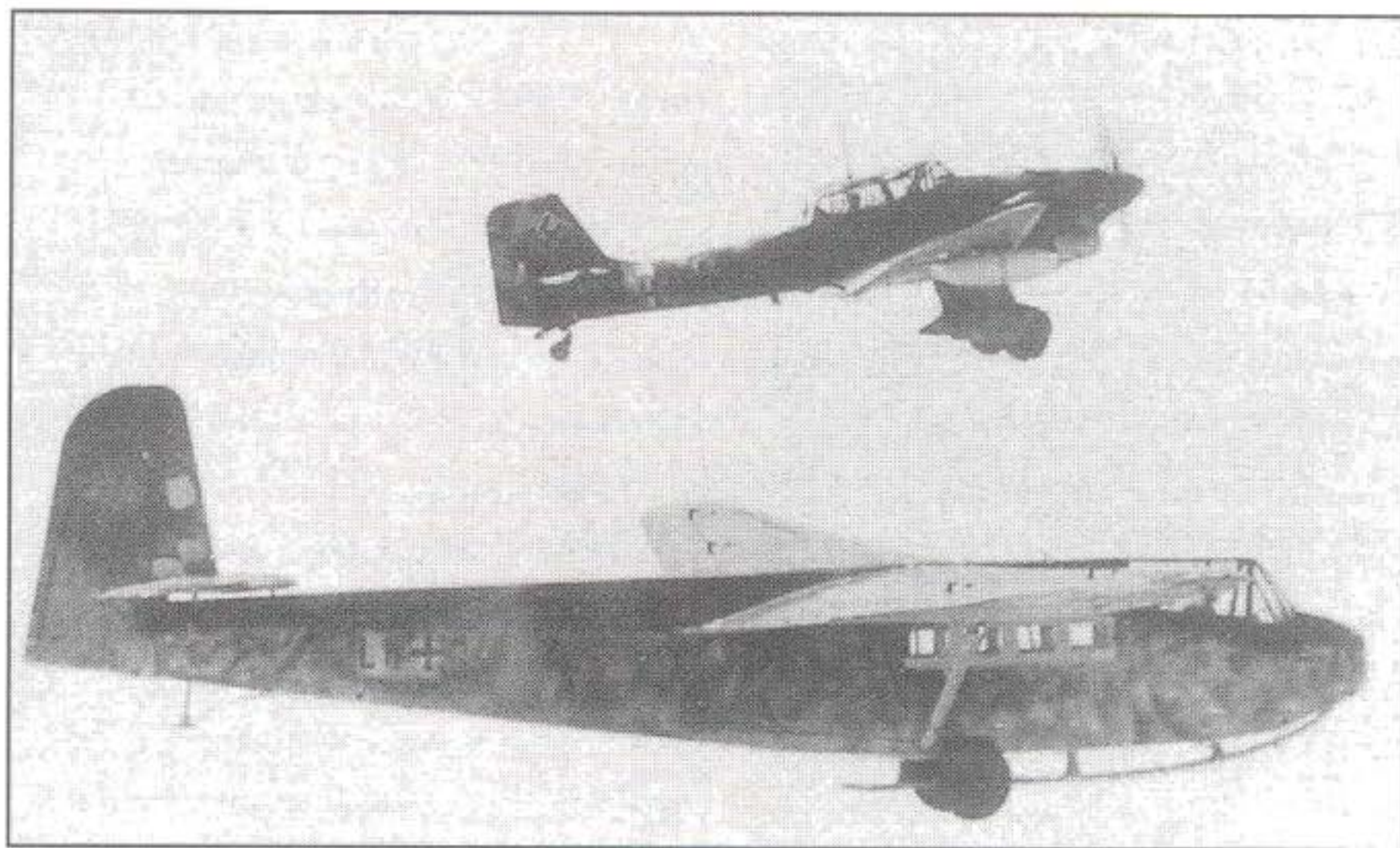
No uncertainty about this Ju 87R. The DFS 230 glider in the foreground and the tow-hook attachment behind the tailwheel clearly identify it as a glider-tug of II./LLG 1
